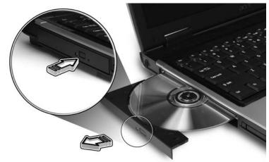
Insert a clip to the emergency eject hole to eject the optical drive tray when the computer is off.
